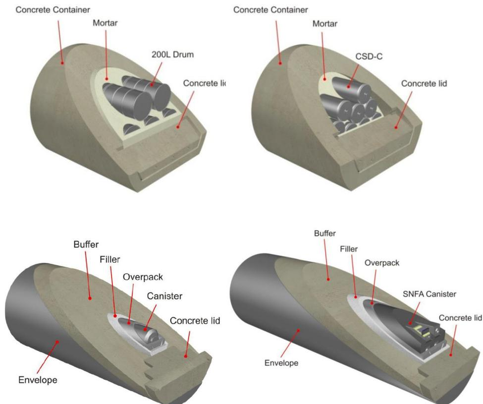
**Monoliths for ILW (top) and supercontainers for HLW and spent fuel (bottom)**
