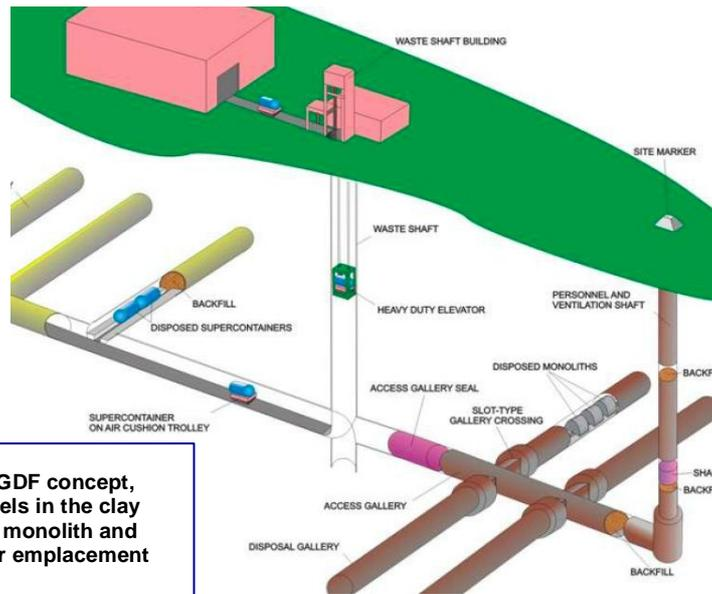
Detail of the GDF concept, showing tunnels in the clay formation for monolith and supercontainer emplacement
