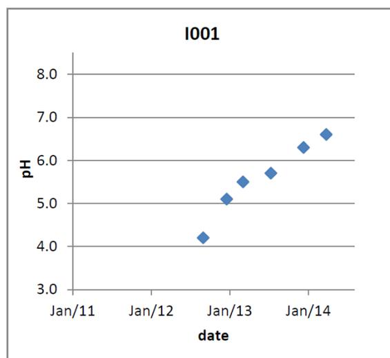
**Figure 3: Oban pH monitored natural attenuation at the trial main injection well (I001) — Source: Aldam, R. (May 2014) *Review of Hydrogeological Conditions Oban ISR Site Havilah Resources NL*, Aldam Geoscience, pg. 41. (Note this report is also in Appendix D of the Final Compliance Report).**
