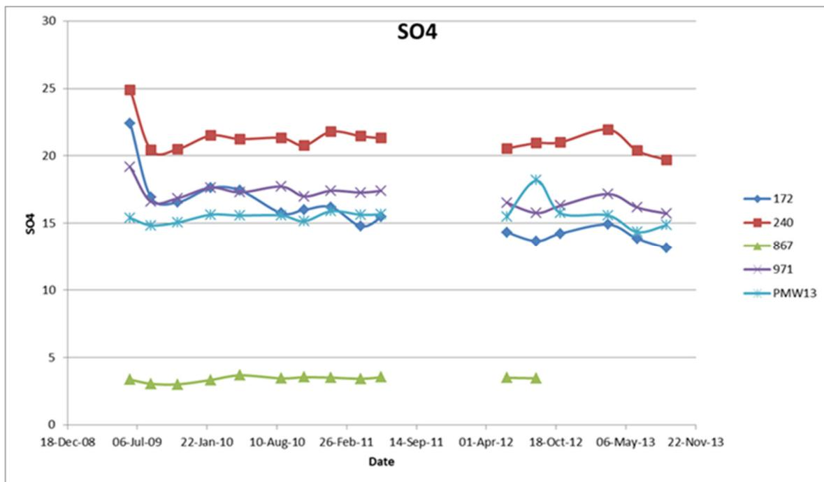
Figure 2: Sulphate (SO4) recovery following cessation of mining activities at selected Beverley wellfield
