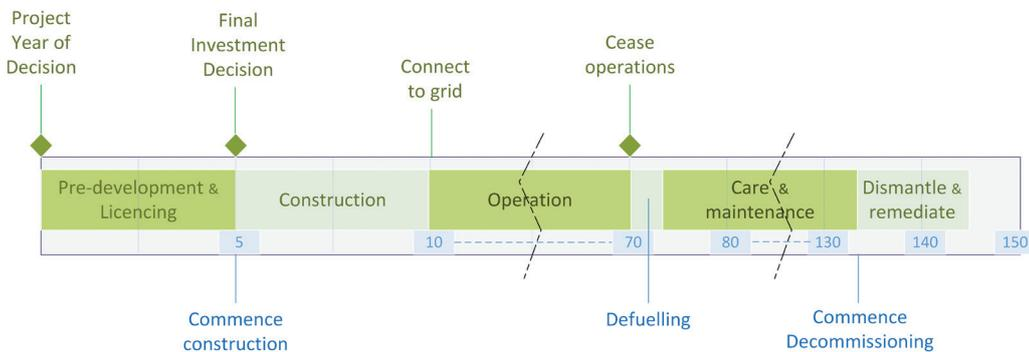
**Figure 1: Assumed nuclear power plant deployment timeline**
