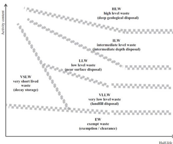
Figure 1: Illustration of the IAEA classification system for radioactive waste
